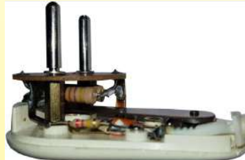
1972 ca. Power control box made by Jidé in Limoges under the brand Jidéstat. The most successful of all systems. Very small in size, it is adjustable, and is incorporated in the electrical plug. This is the only model with a snap magnet contact. It was not surpassed by electromechanical systems until the current era. (Ultimheat Collection)
