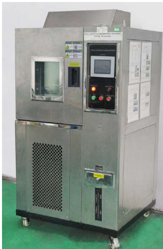
Climate chamber, with temperature adjustment range from -90 to +150^\circ\text{C} , relative humidity adjustment range 1 to 100%
