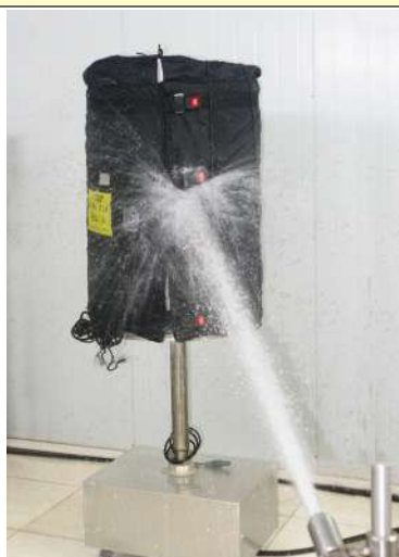
IPx6 testing of jacket heaters
