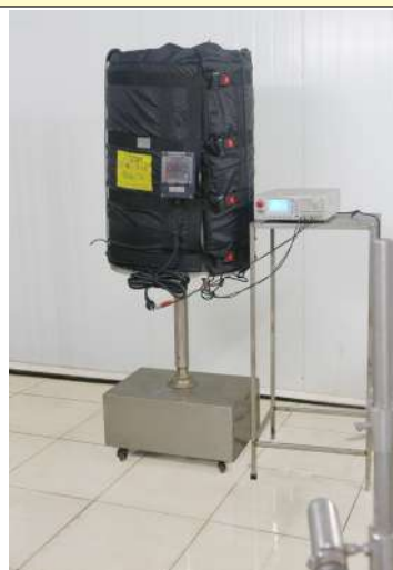
Insulation resistance measurement after IPx6 tests
