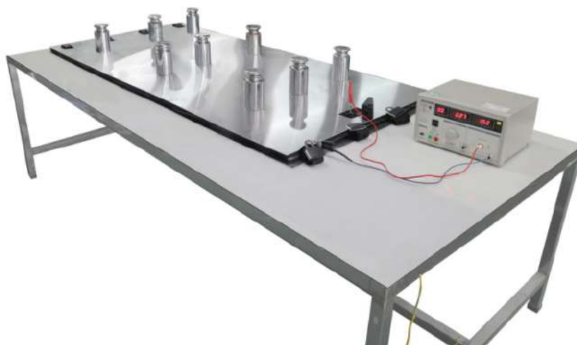
Measuring equipment for total current leakage at cold condition
