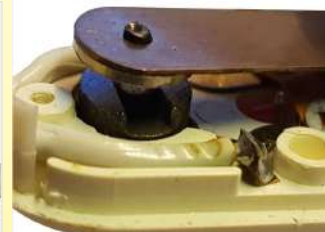
1972 ca. Power control box made by Jidé in Limoges under the brand Jidéstat. The most successful of all systems. Very small in size, it is adjustable, and is incorporated in the electrical plug. This is the only model with a snap magnet contact. It was not surpassed by electromechanical systems until the current era. (Ultimheat Collection)
